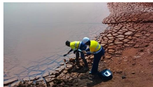
Figure 34: Onsite water quality test using Horiba Meter at Sediment Retention Pond 4 at Naibulu Mine Site.
