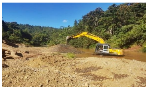
Figure 33: Excavator extracting from the mid-river, which is not allowed.
