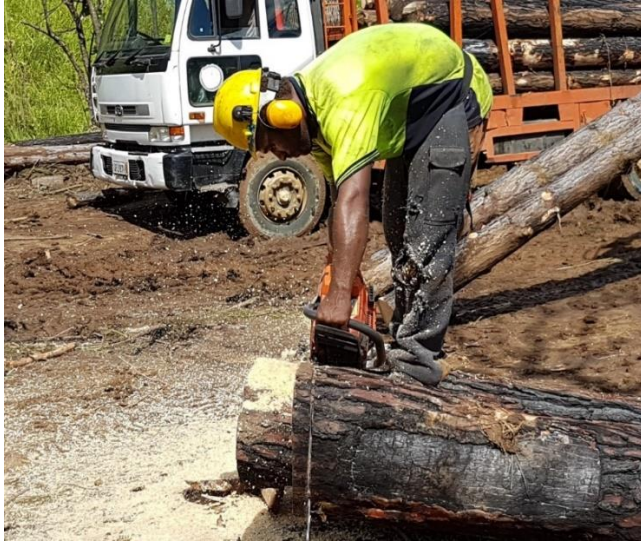
Cutting of Density Discs from a Tapped Pine log
