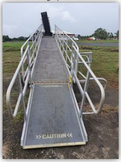
Figure 5.102: Mechanical ramps used for boarding larger planes
