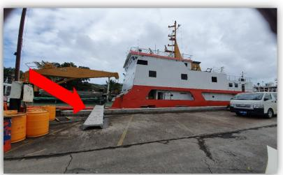
Figure 5.56: Steel boards used for boarding by Conventional Motor Vessels
