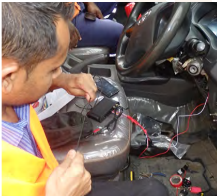
FEA installed Vehicle Tracking System in 2015 in all the FEA vehicles to specifically assist in maintaining safe speeds and highlighting over speeding breaches as well as abuse of vehicle usage and management of fuel efficiency.
