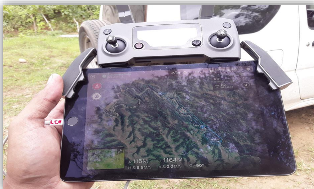
Figure 5.4: Route of drone mapped to follow and current image display
