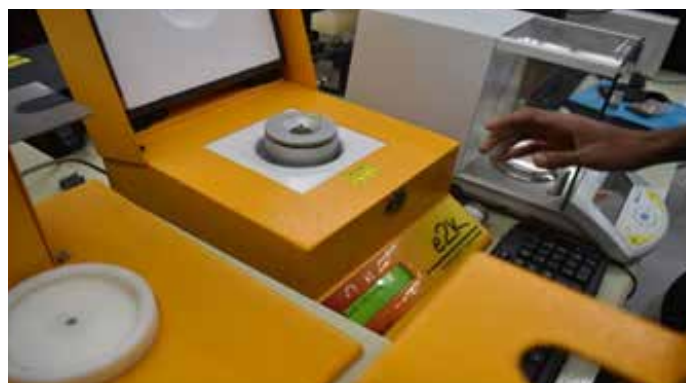
Insertion of the capsule (which contains the sample) in the combustion calorimeter.
