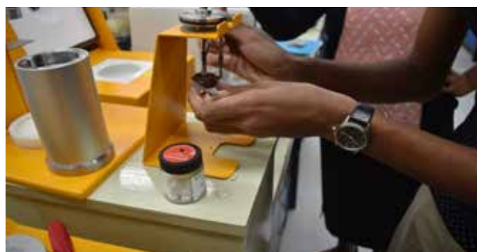
Connecting the firing wire to the sample.
