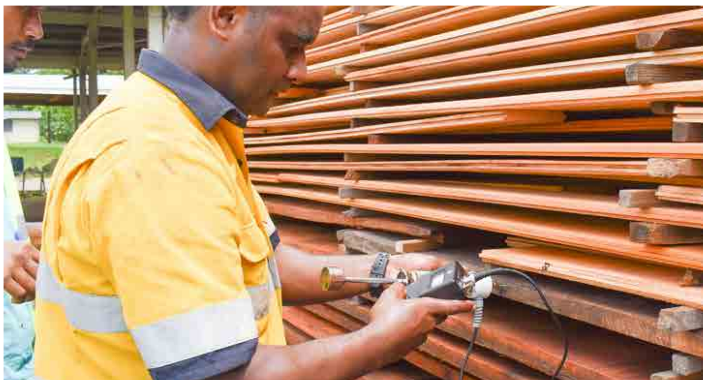
Moisture content assessment for kiln dried timbers
