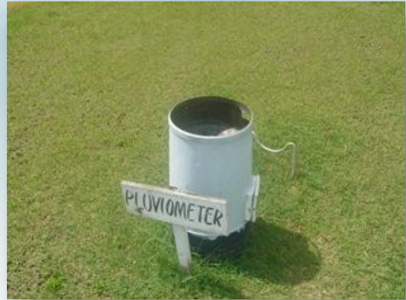
Figure 1: Pluviometer - measures time and intensity of rainfall
