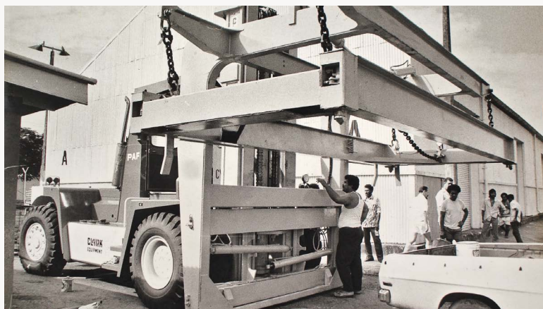
With a lifting capacity of a massive 65,000lb, these were the first of their kind container handling equipment ordered by Ports Authority of Fiji to meet the large number of containers then coming into Fiji.
