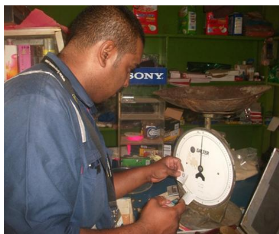
Assistant Inspector, stamping a salter 10kg scale
