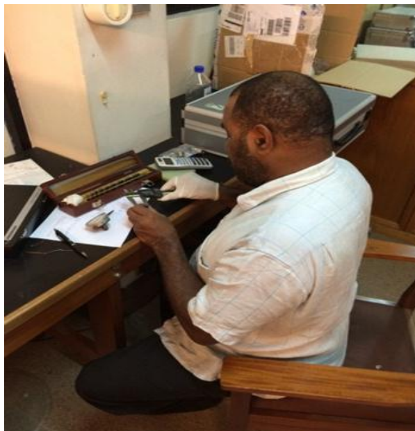
Verifying a Venier clipper on a certified gauge
