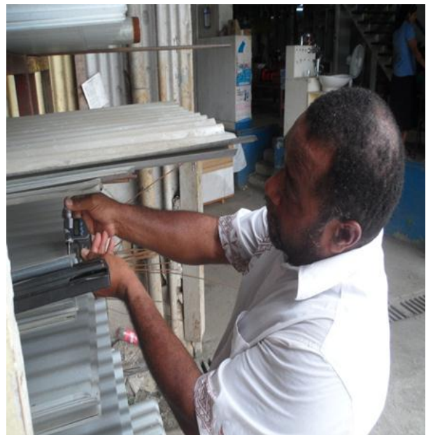
Assistant Inspection of the thickness of the roofing coils block using a Micrometer
