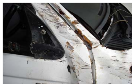
Close-up view of EM866, bona-fill is evident. Bona-fill is used when a vehicle has an accident
