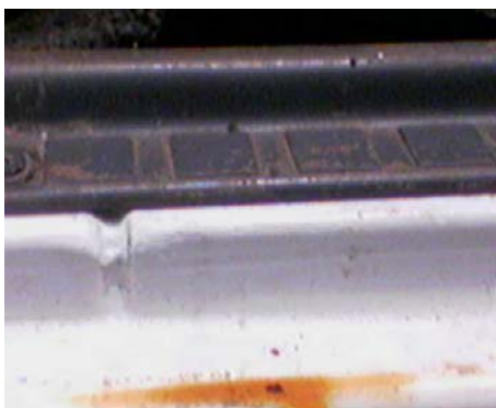
The rusted door step of GM549 as at April, 2007
