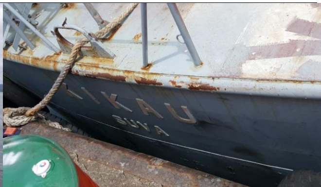
Stern (aft-most / rear side) of RFNS Vessel Kikau rusting and not painted by contractor A
