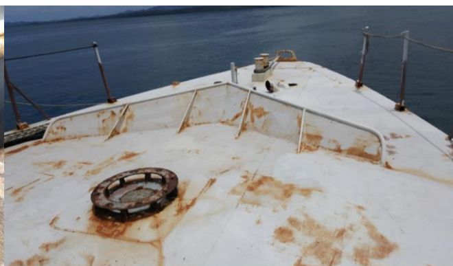
Bow (front deck) of RFNS Vessel Kikau showing painting works not done by the contractor A
