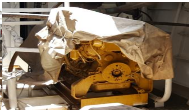
Generator of RFNF Vessel Kikau; has not been fully installed to the vessel by Contractor A
